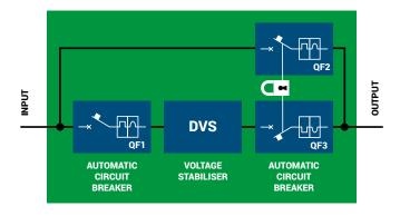
QF3 is interlocked with QF2 by means of an individual key. When one of the breakers is closed, the other one is open and the closing spring cannot be manually loaded.
