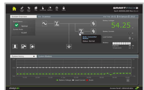
STATUS OF DC/DC CONVERTERS IN SMARTPACK2 WEB
